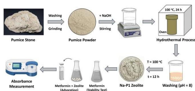
Figure 1 depicts a simplified zeolite synthesis technique
