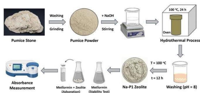
Figure 1 depicts a simplified zeolite synthesis technique
