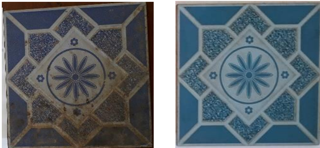
Figure 2. Comparison of ceramic samples: (a) dirty ceramics that are difficult to clean, (b) ceramics that have been cleaned with a floor-cleaning formula
